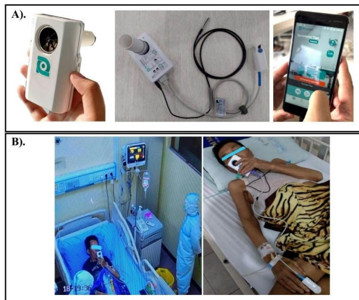
Figure 1. A). RESPINOS remote monitoring device. B). The implementation of RESPINOS to measure the vital signs of COVID-19 patients.
