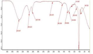
Figure 5 FT-IR spectra showing presence of different functional groups engaged in synthesis of nanoparticles
