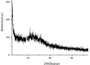
Figure 6 XRD spectra showing diffraction pattern of synthesized nanoparticles.
