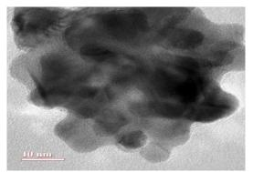
Figutre 4 The internal size of synthesized nanoparticles using TEM
