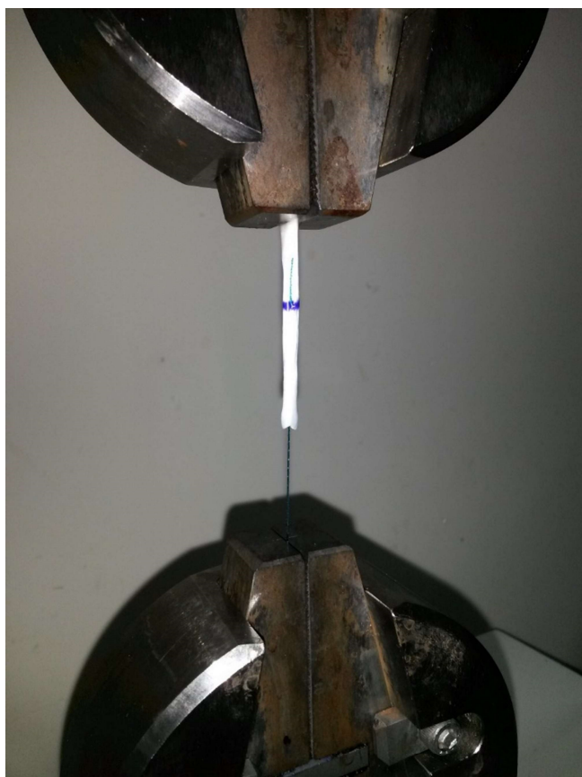
Figure 3: A photo showing a specimen from group 3 while being tested for ultimate tensile strength.
