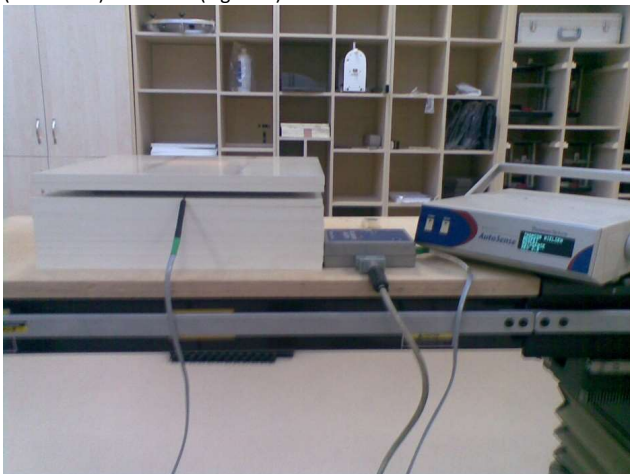
Figure 1.The set-up of Mosfet AutoSense system
