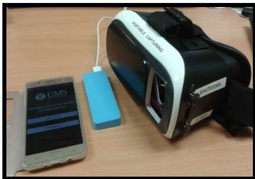
Figure1. PSCN has two components: The goggle and the developed (APPs) downloaded in the smartphone. A power bank is used for charging the system.PSCN: Portable System for Capturing Nystagmus. APPs: an application software.
